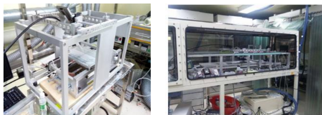
Figure 3: (Left) 30 cm automatic blade coater (Right) 120 cm coater under assembly
